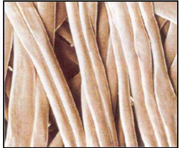
Magnified view of the fabric of "Zemdrain" Permeable Membrane
