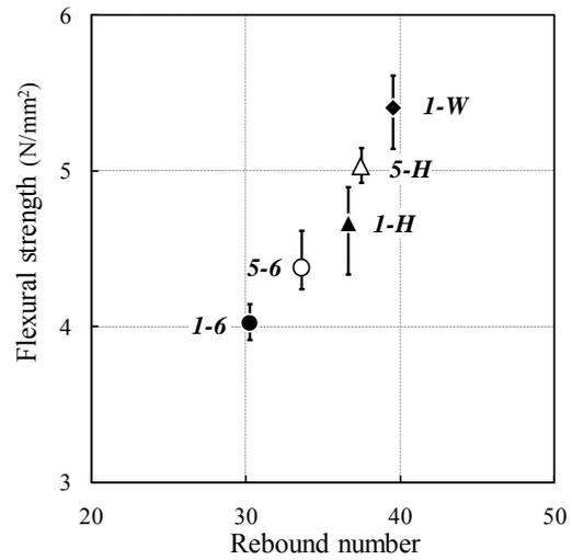
Figure 6. Relationships between rebound number and flexural strength
