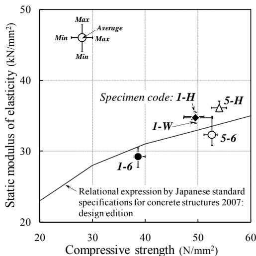
Figure 1. Effects of curing conditions on compressive strength and static modulus of elasticity
