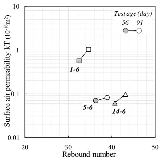
Figure 11. Effects of demold age on surface air permeability or rebound number of the specimens exposed to 60%RH air
