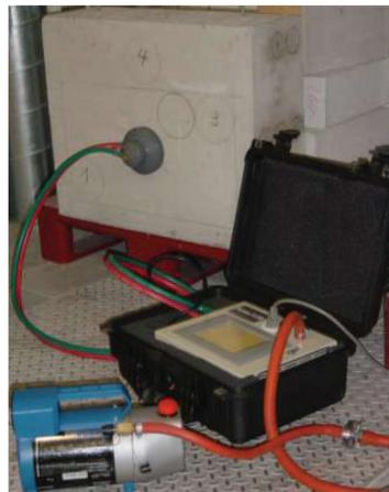
Figure 2. Application of site air-permeability test on “F” surface of the panel.
