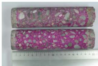
Figure 4. Carbonation of “Z” (left) and “F” (right) faces.
