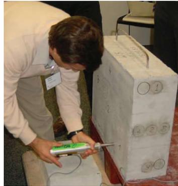
Figure 1. Application of Rebound Hammer on “Z” surface of the panel.
