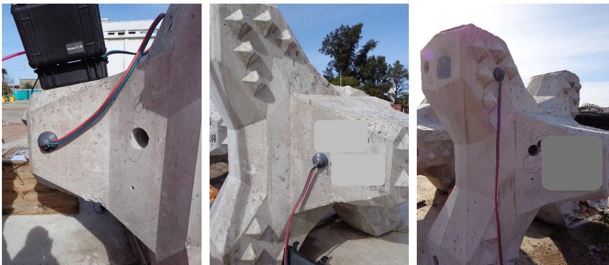
Fig. 5 - a) Tests performed on broken element
