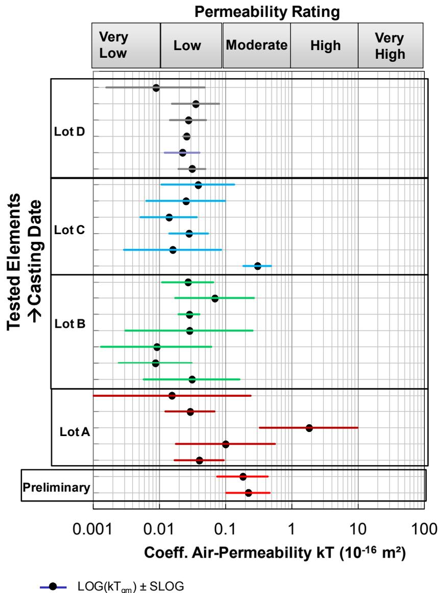
Fig. 6 - Mean and scatter of results obtained on the Accropodes<sup>TM</sup> II tested
