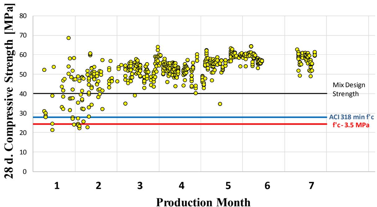
Fig. 3 - 28-day Compressive Strength of 1129 concrete samples
