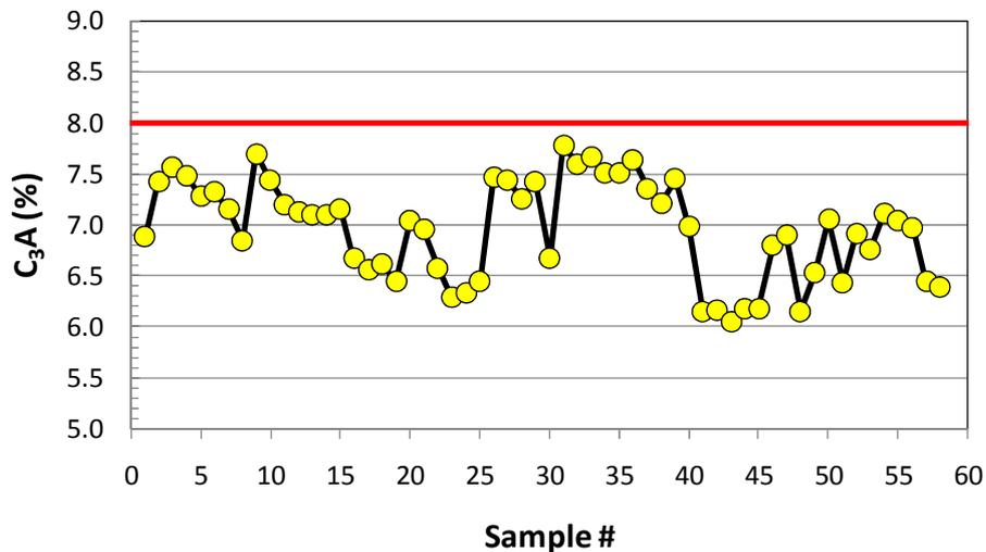
Fig. 2 - Variation of  $C_3A$  content of 58 cement samples
