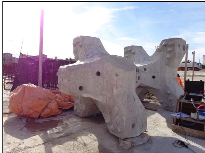
Fig. 4 - Preselected Accropodes™ II (broken element at the foreground) ready for testing
