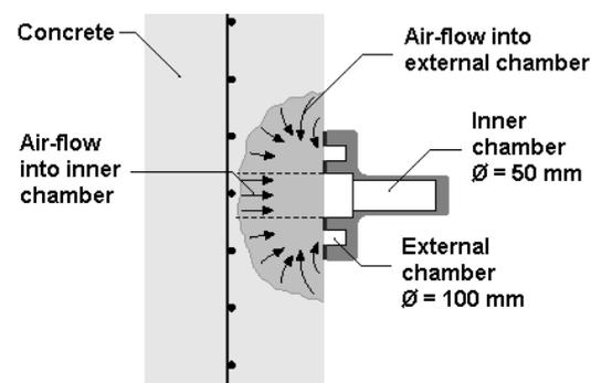
Fig. 7 – Sketch of air-permeability test.
